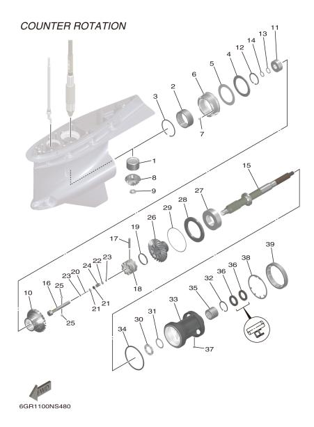
FIG. 47 LOWER CASING & DRIVE 5
