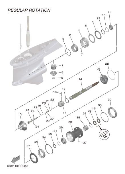
FIG. 44 LOWER CASING & DRIVE 2
