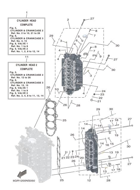
FIG. 5 CYLINDER & CRANKCASE 2
