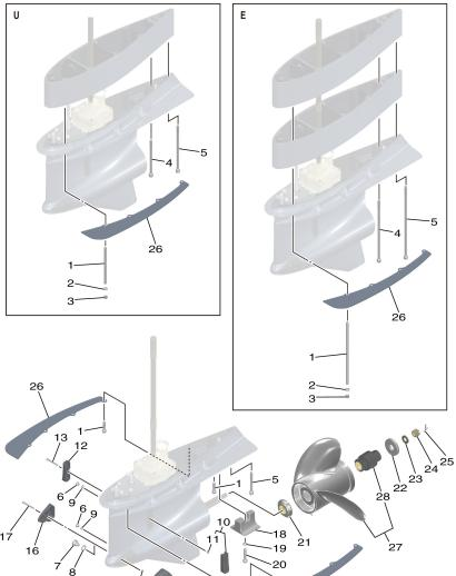
FIG. 45 LOWER CASING & DRIVE 3
