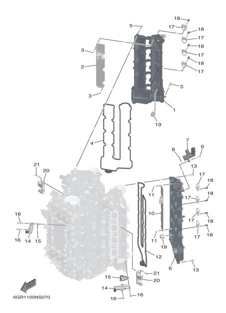
FIG. 6 CYLINDER & CRANKCASE 3
