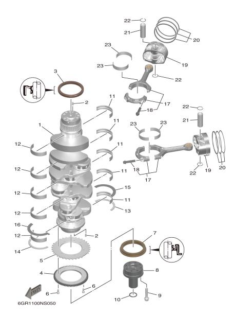
FIG. 4 CRANKSHAFT & PISTON
