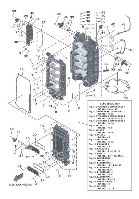
FIG. 3 CYLINDER & CRANKCASE 1
