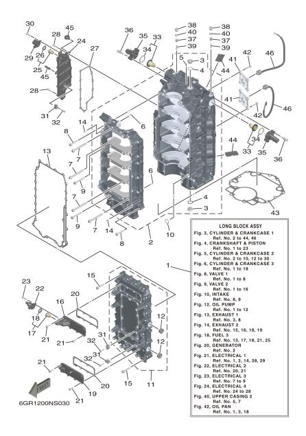
FIG. 3 CYLINDER & CRANKCASE 1
