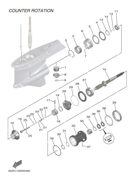
FIG. 47 LOWER CASING & DRIVE 5
