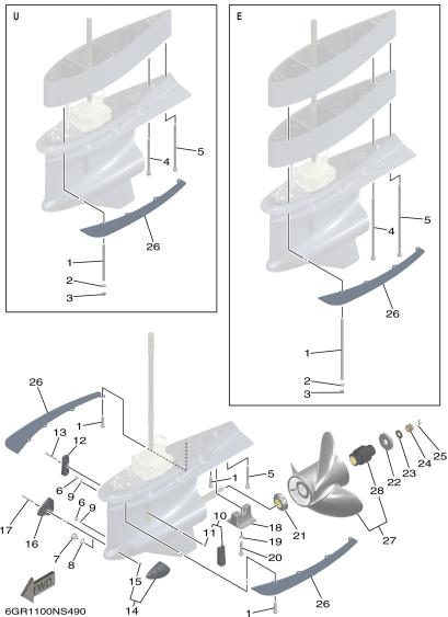
FIG. 48 LOWER CASING & DRIVE 6
