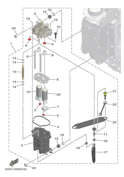
FIG. 15 VAPOR SEPARATOR
