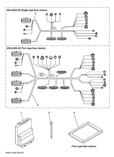
FIG. 7 ELECTRICAL DBW REMOTE CONTROL
