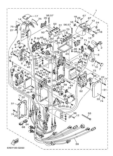
FIG. 5 DBW REMOTE CONTROL 2 (TWIN)
