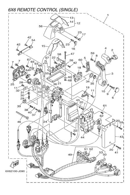
FIG. 9 DBW REMOTE CONTROL 1 (SINGLE)
