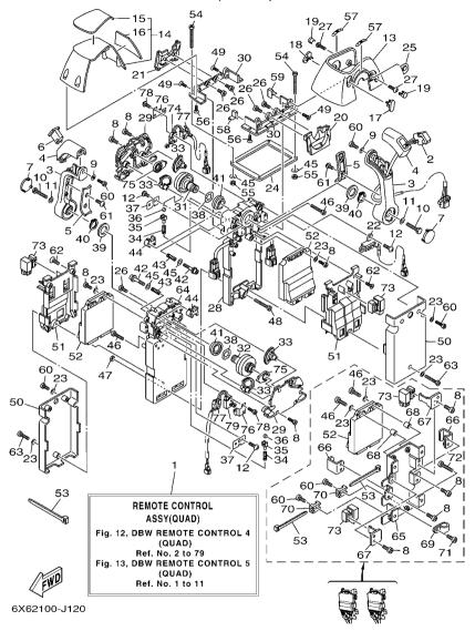
FIG. 12 DBW REMOTE CONTROL 4 (QUAD)
