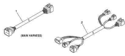
Uses to connect between main helm RC and 2nd hlem RC.
