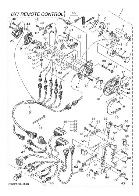
FIG. 14 DBW REMOTE CONTROL 6 (6X7)
