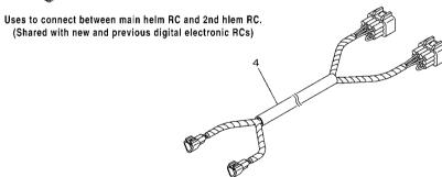
Uses to connect between main helm RC and 2nd hlem RC. (Quad RC special)
