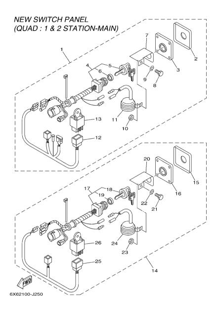
FIG. 25 SWITCH & PANEL 11 (QUAD)
