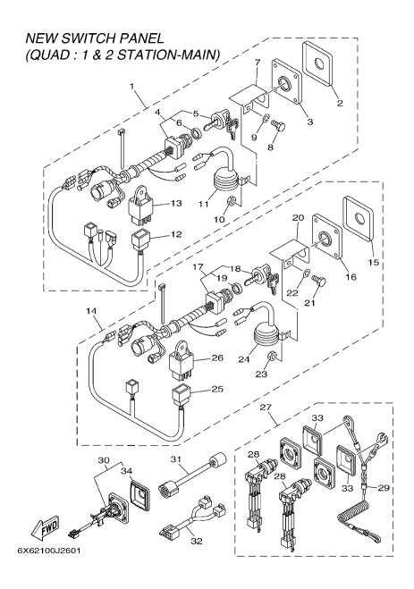
FIG. 26 SWITCH & PANEL 12 (QUAD)
