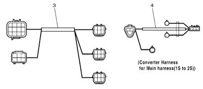
(2S Converter Harness for current Triple Switch panel-New control Box)
