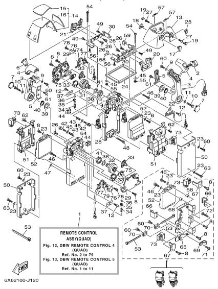
FIG. 12 DBW REMOTE CONTROL 4 (QUAD)
