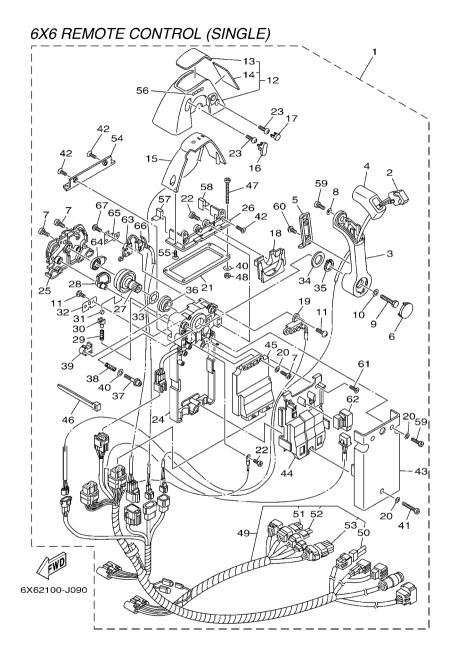
FIG. 9 DBW REMOTE CONTROL 1 (SINGLE)
