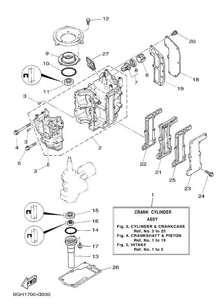
FIG. 3 CYLINDER & CRANKCASE
