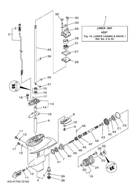
FIG. 16 LOWER CASING & DRIVE 1
